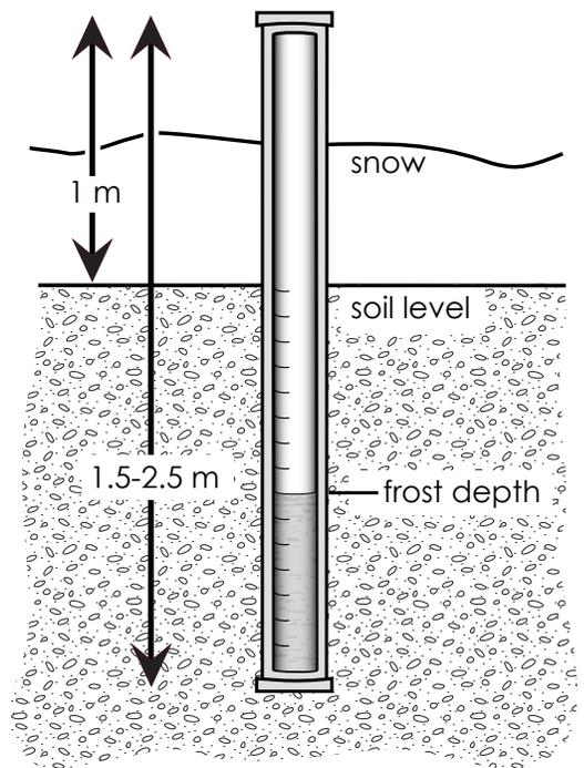
7. Frost depth should be measured on the same day at the same time each week, ideally within one hour of solar noon. To measure, remove the cap on the CPVC pipe and raise the flexible inner tube.
